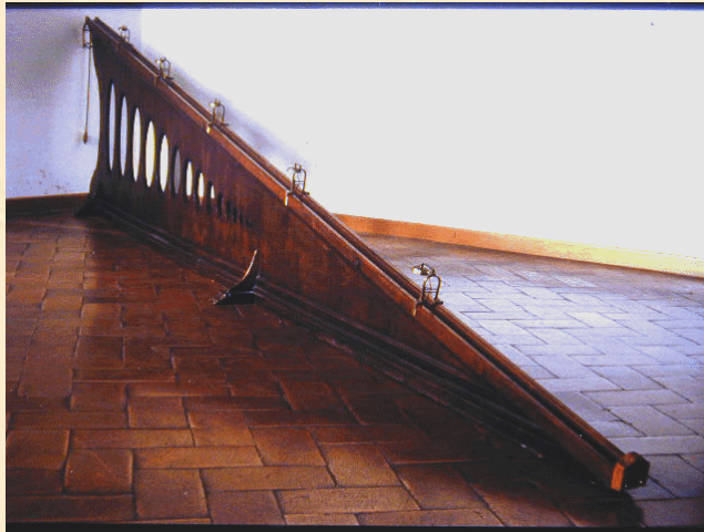
Galilei's inclined plane
