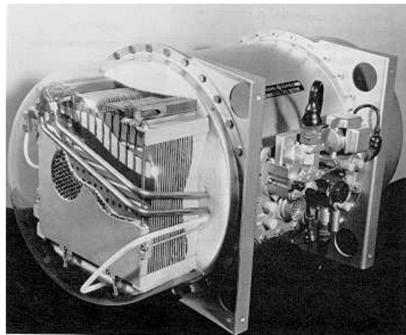
Most current models use natural gas to supply hydrogen, such as this model for refrigerated trucks.
