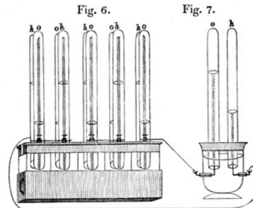
**In the hydrogen-oxygen fuel cell, hydrogen is fed to one porous electrode and oxygen to the other. The electrodes are separated by an electrolytic material.**
