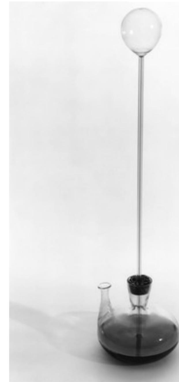
These first thermometers were sensitive to air pressure, and worked as much as a barometer as they did as a thermometer.
