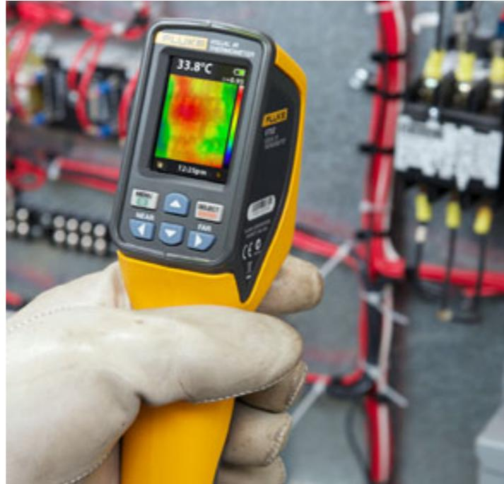
**IR thermometers are used by firefighters to detect hot spots in buildings, restaurants to ensure that served food is still hot, and wherever a quick surface temperature is needed.**
