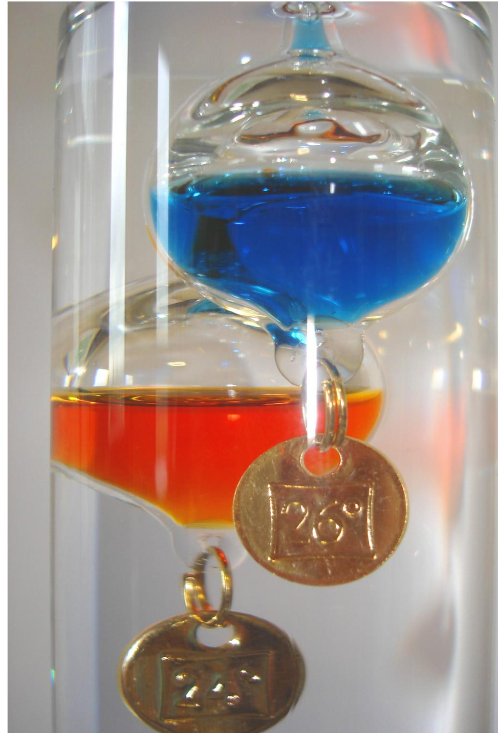
**The liquid within each glass sphere is composed of either colored water or alcohol.**
