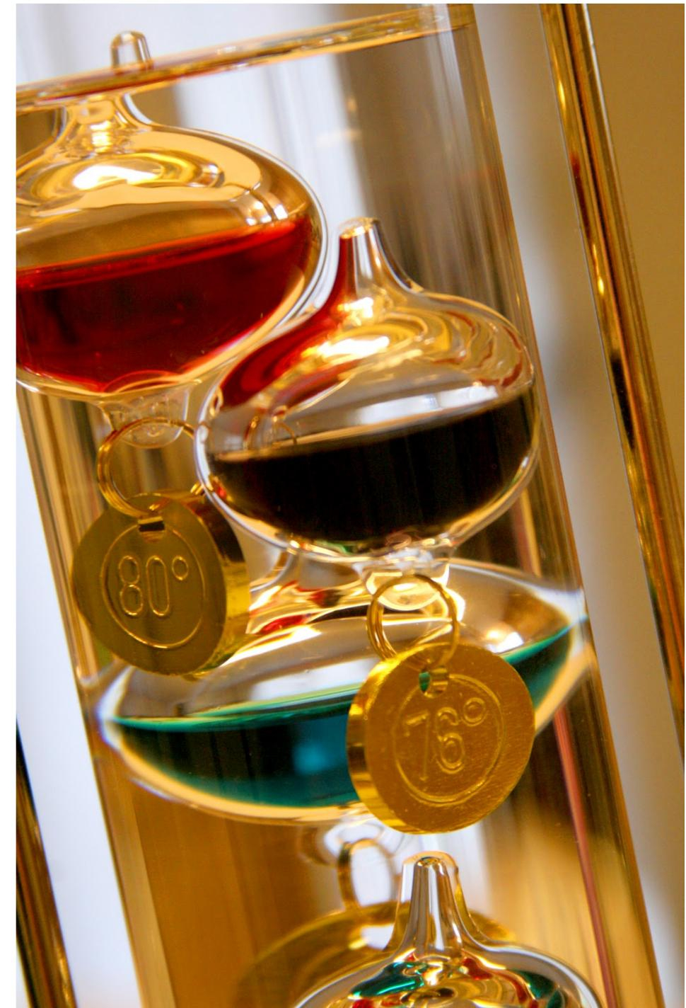
Even though they look nothing like a “normal” thermometer, the Galileo thermometer still functions according to the same basic principle as most other thermometers: substances expand when heated and contract when cooled.
