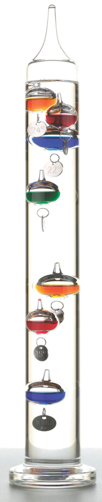
Attached to each of the colored spheres is a little dangling metal tag with an engraved temperature.
