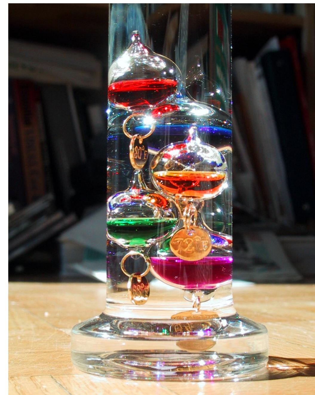
**As the oil warms, it expands, becomes less dense, exerts a smaller buoyant force, so the heaviest sphere sinks.**
