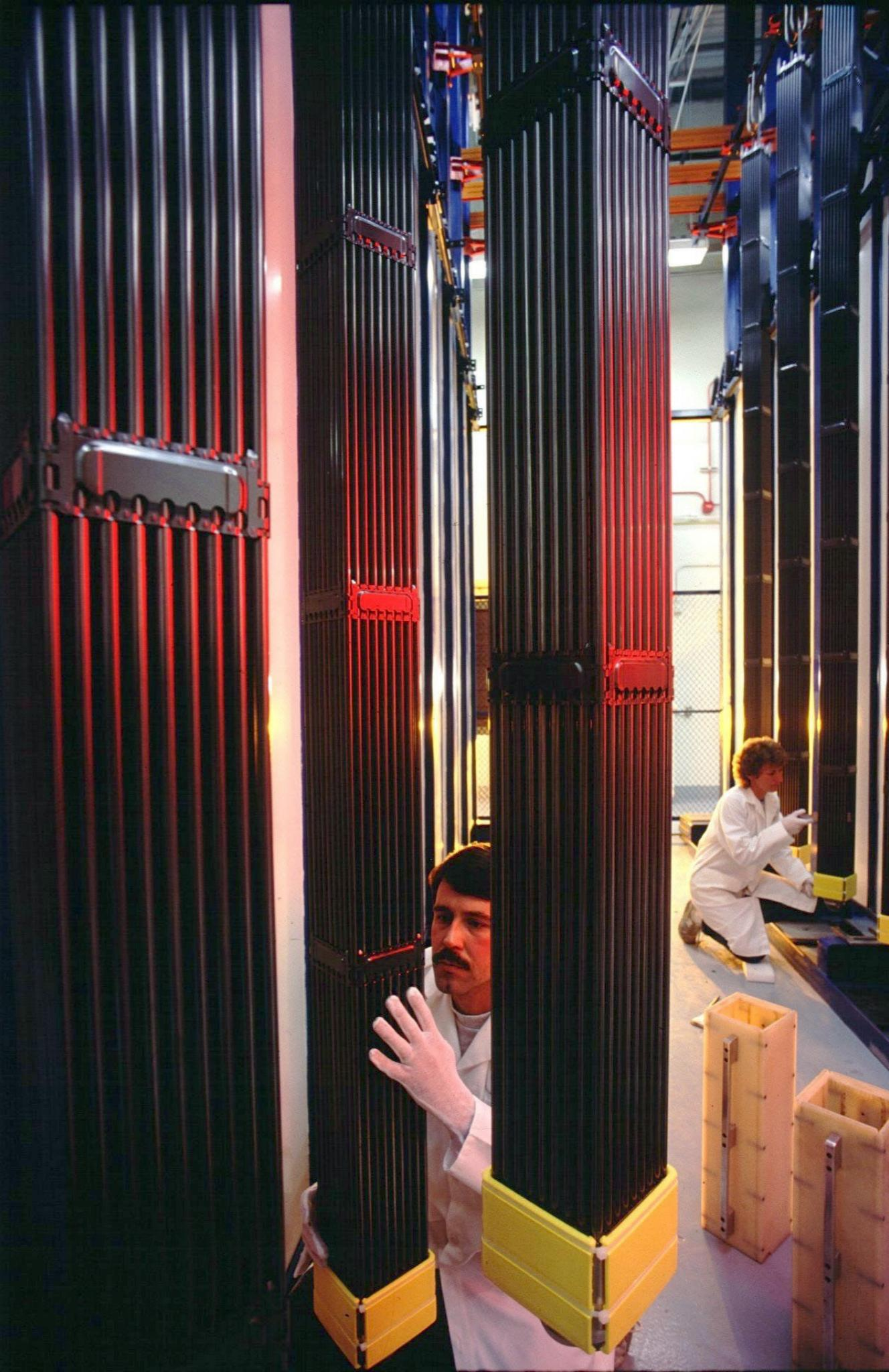
**Rods contain pellets of uranium enriched to ~3%  $^{235}\text{U}$ .**
