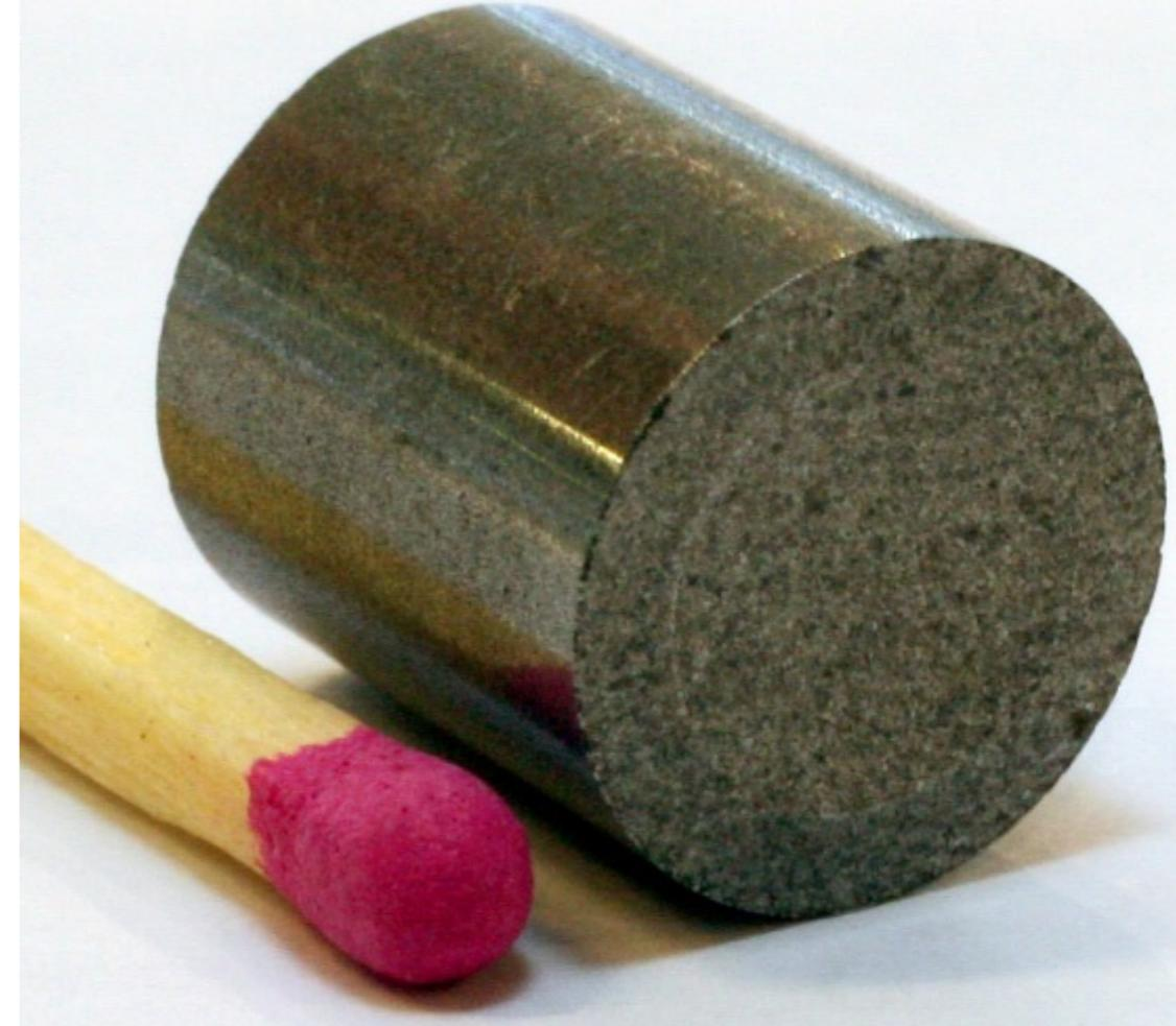
**With an energy of 10 trillion J/kg, one needs ~10,000 kg/yr of pellets for 1 GW of electrical power.**
