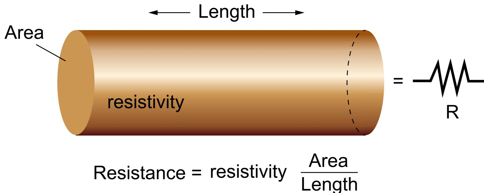
**All copper has the same resistivity, but a 2m copper wire has twice the resistance of a 1 m copper wire of the same diameter.**
