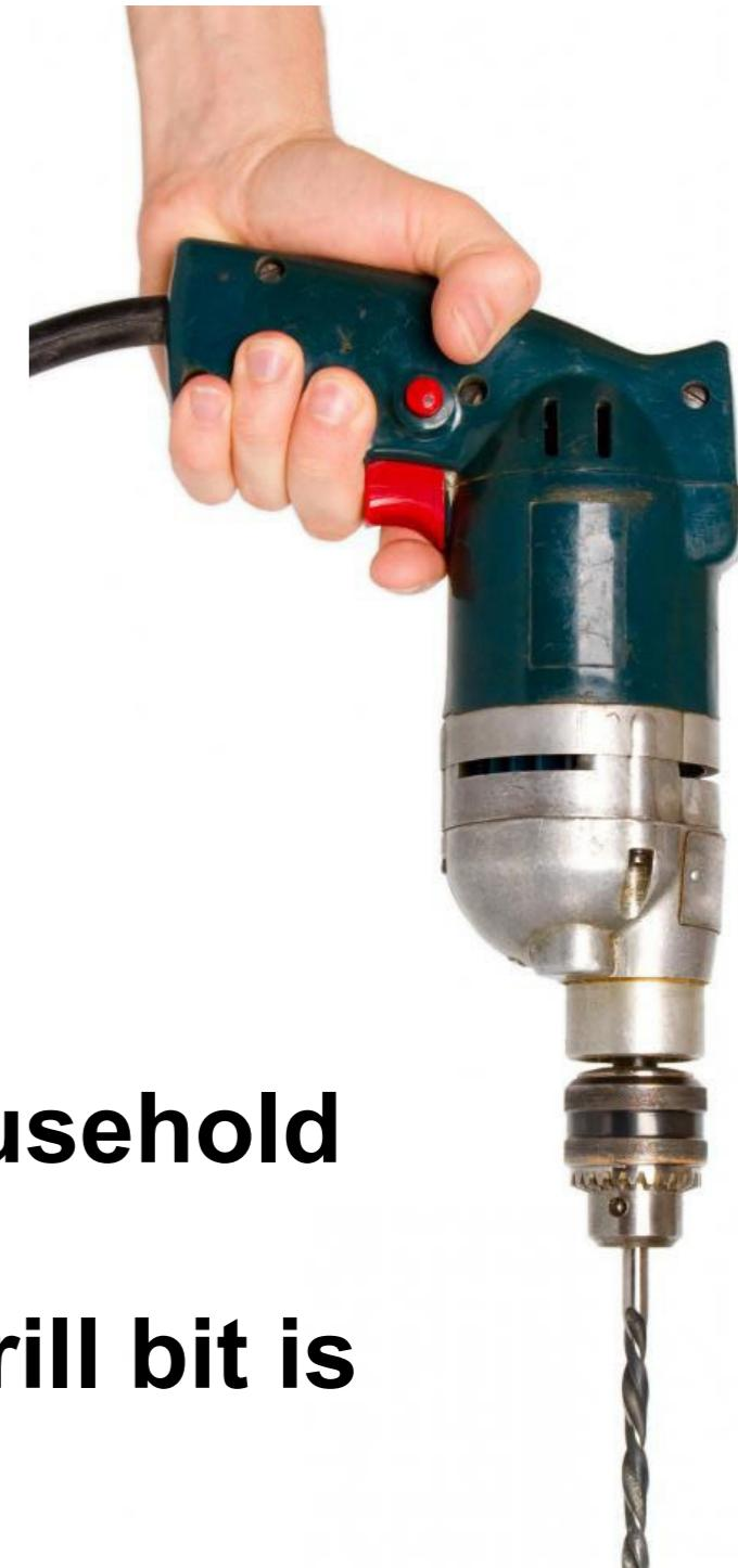
**An electric drill connected to a household 120 V source draws 2 A of current. The power being supplied to the drill bit is  $120V \times 2 A = 240 W$ .**
