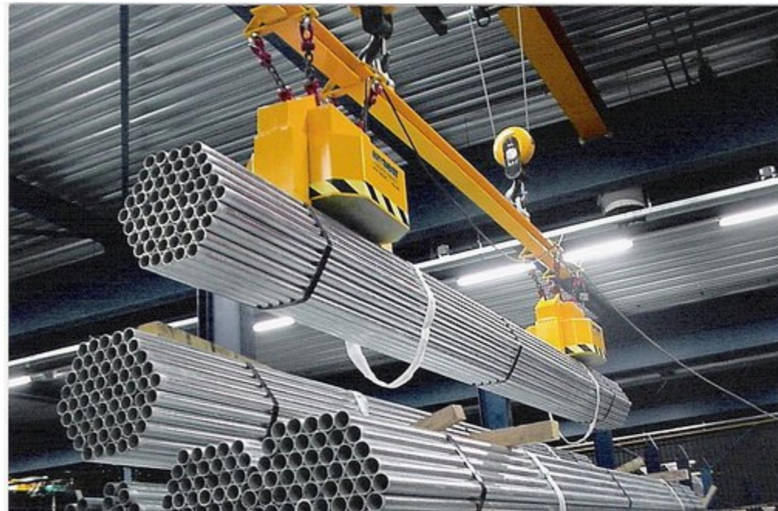
**When the current is turned off, the piece of iron will return to its random magnetic orientation.**
