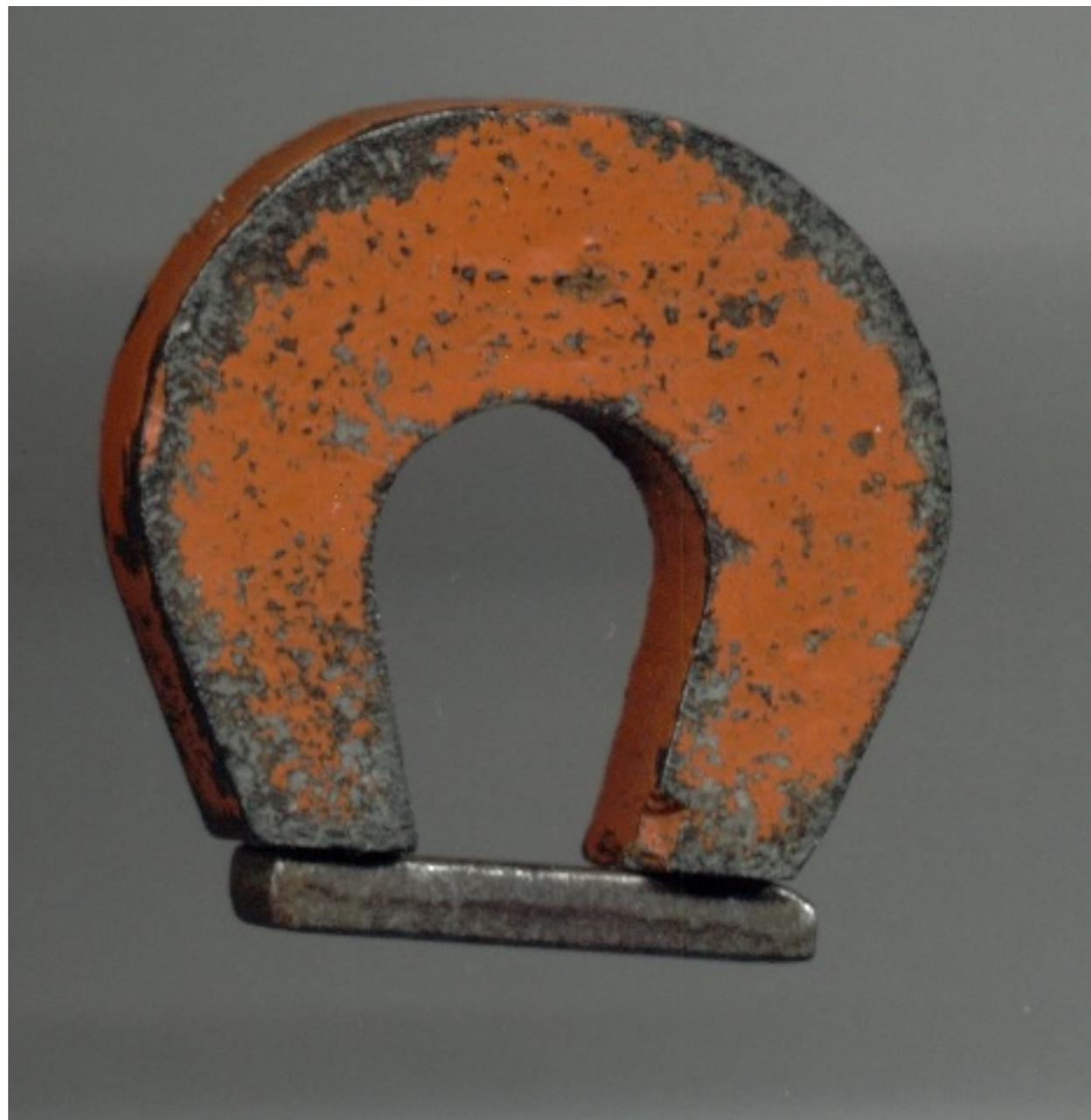
**In materials known as ferromagnets - iron for example - these little magnetic fields can line up in the same direction to give a macroscopic magnet.**
