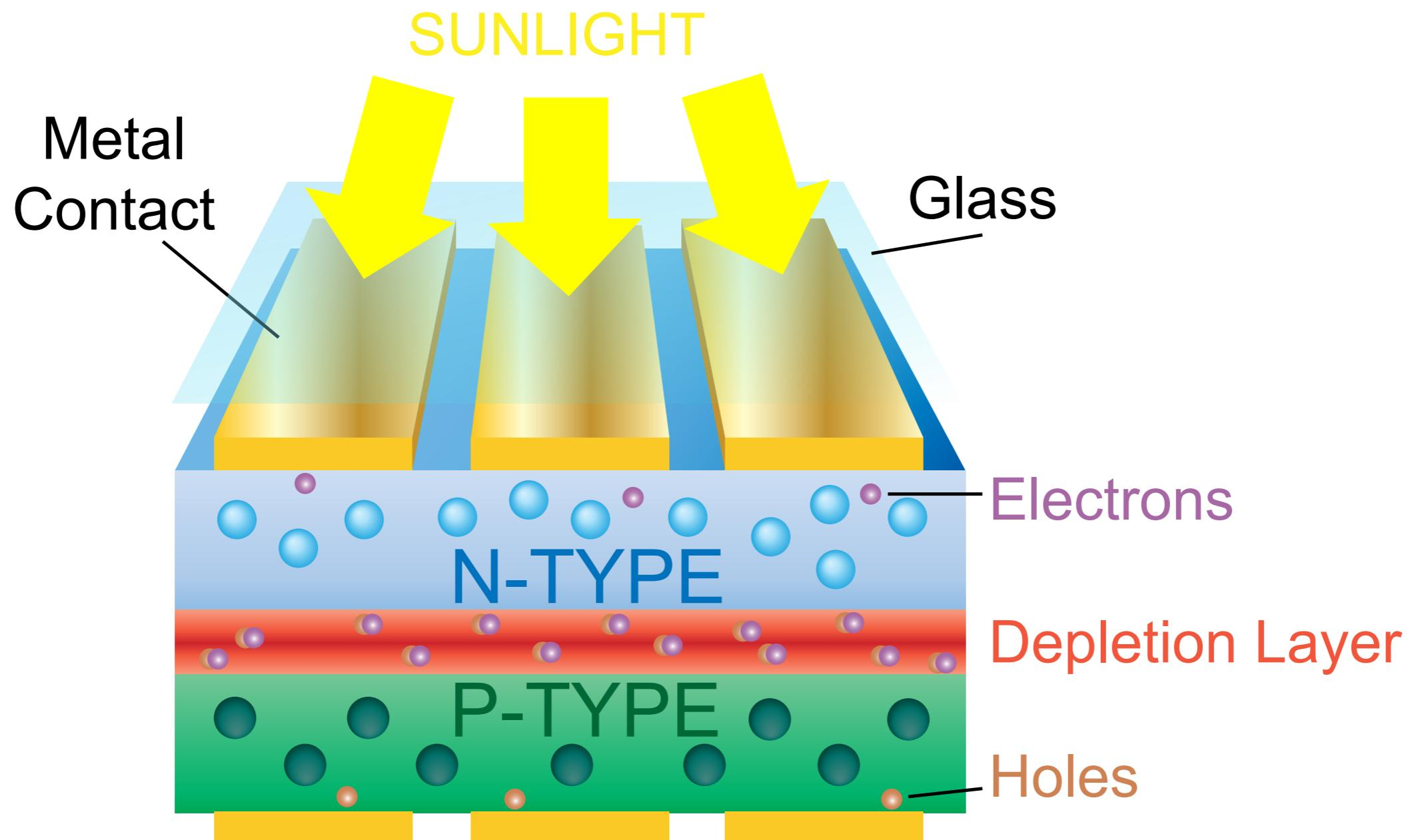
The electron flow provides the DC current, and the cell's built-in electric field causes a voltage.
