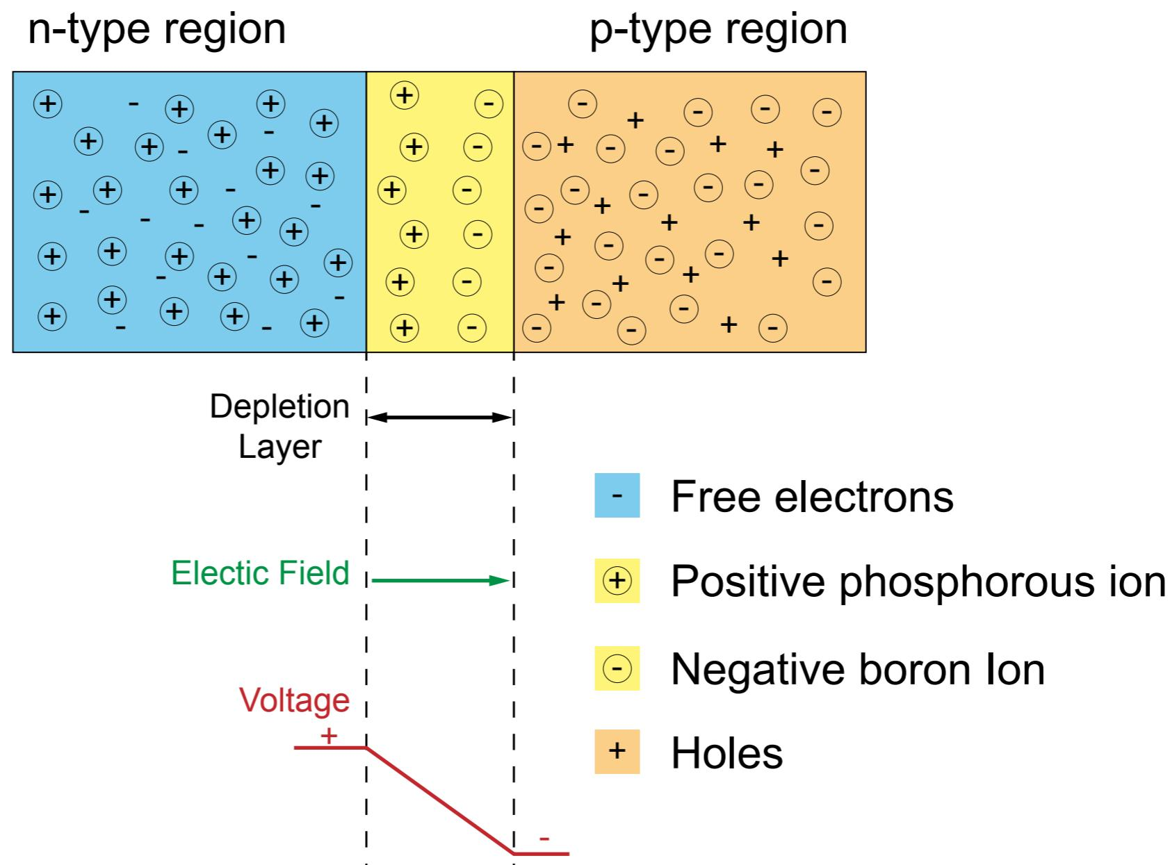
If this happens close to the built-in electric field, the field will send the electron to the N side and the hole to the P side.
