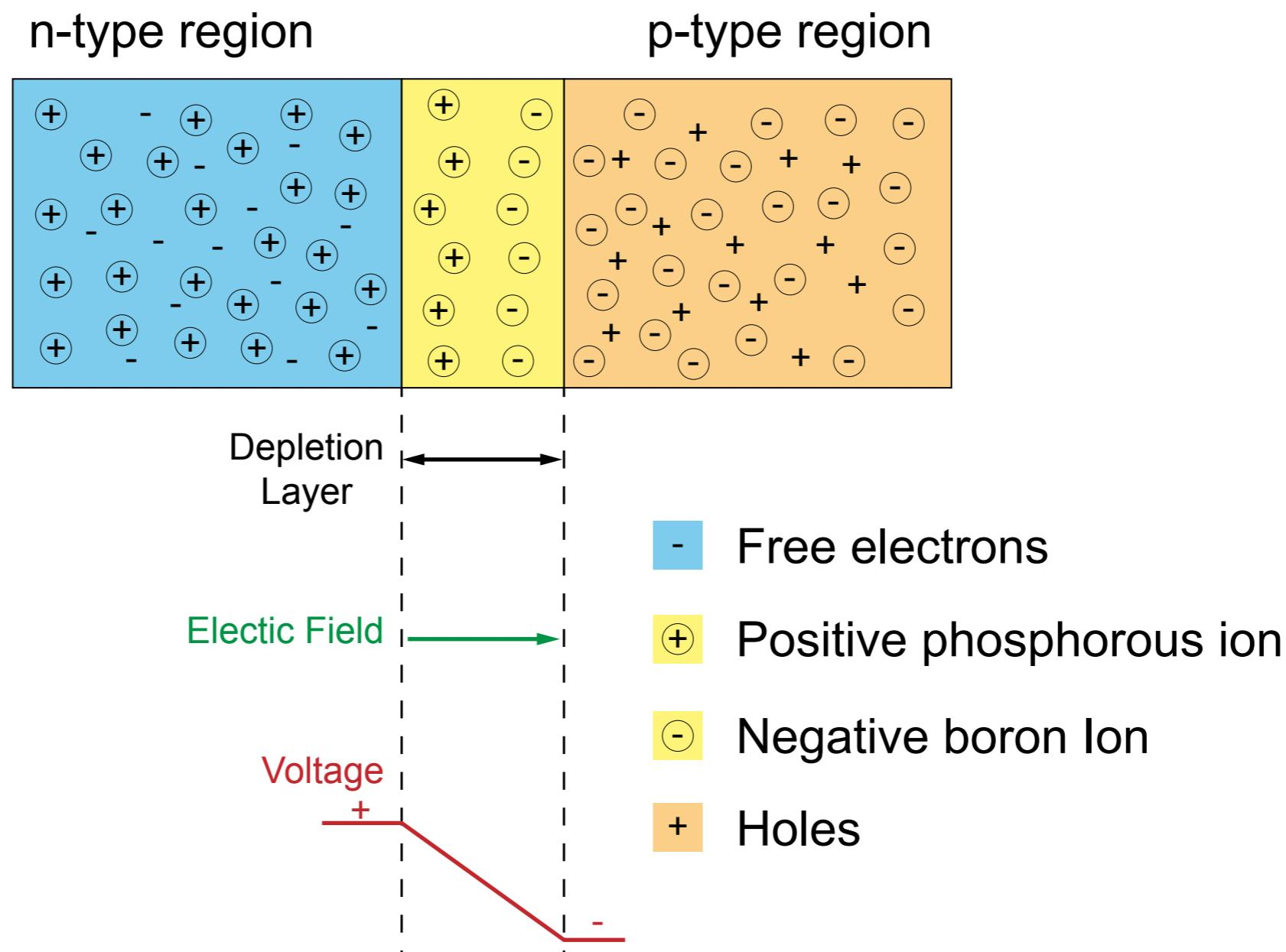
It's like a hill - electrons can easily go down the hill (to the N side), but can't climb it (to the P side).
