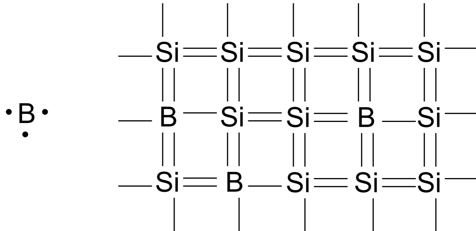
**Silicon with such impurities is called “p-type”, with the “p” signifying the extra positively charged openings (holes).**
