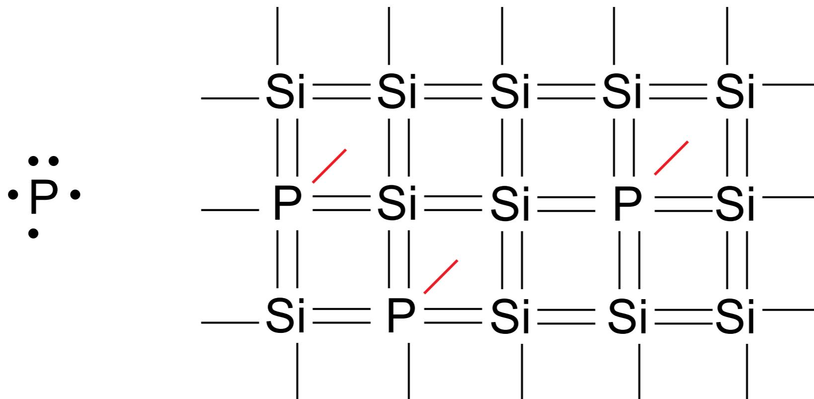
Silicon with such impurities is called “n-type”, with the “n” signifying the negatively charged electron.
