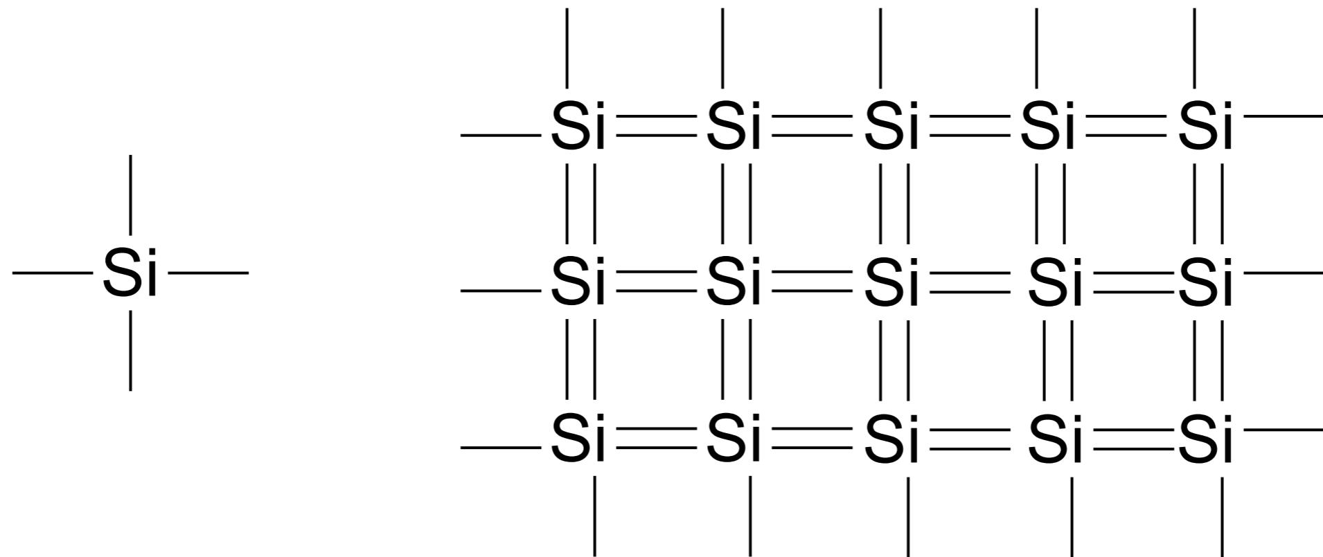
**A silicon atom will always look for ways to fill up its last shell, and to do this, it will share electrons with four nearby atoms. This is what forms the pure silicon crystalline structure.**
