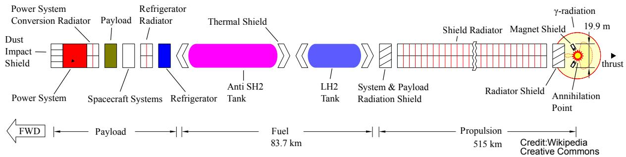
Storing antimatter for use in a rocket is especially challenging because if it touches any matter whatsoever, well, you'll have quite the explosion. Folks have considered magnetic bottles, but the bottle has to be 100% empty of ordinary matter. Otherwise, Bang!
