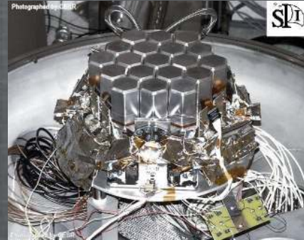
INTEGRAL's coded-mask spectrometer with a 19-element Germanium solid-state detector.
