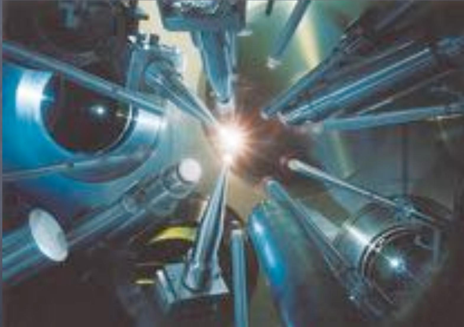
A millimeter-wide pellet of hydrogen explodes under the multiple-angled fire of the Omega laser during a recent experiment at the Laboratory for Laser Energetics.
