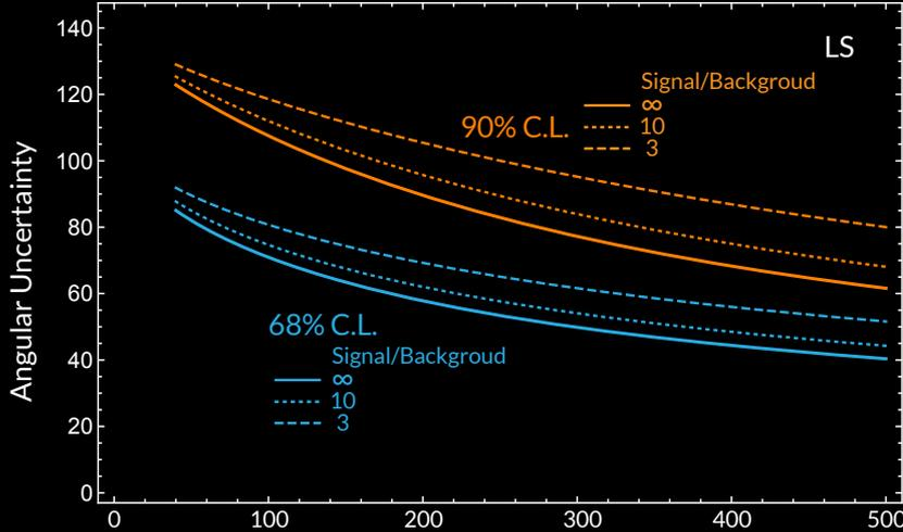
Enhanced liquid scintillators could localize a pre-supernova to  $\sim 15^\circ$  at 90% confidence after  $\sim 200$  detections.
